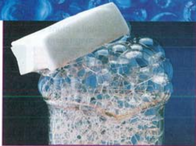
This white aerogel has such a low density that it can float on top of soap bubbles.
